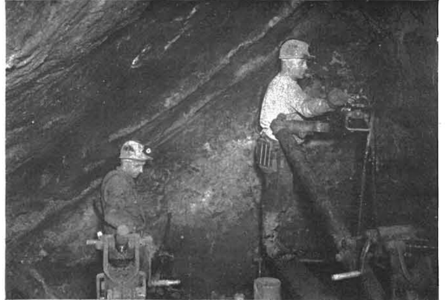
Drift miners Harold Wills and John Kipina, operating drilling machines from a "jumbo."
